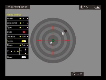
2. On the frozen image, move the green "x" mark along the X-axis and Y-axis until the "x" mark is precisely aligned with the initial shot's point of impact.
