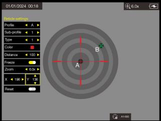
3. The reticle has been zeroed. Save the position as a profile. The user can save and recall up to 25 different ballistic profiles.
